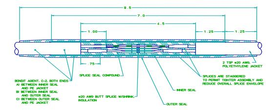
The **Sealing Compound** encapsulates the electrical splices, provides a strain relief for the conductors, acts as a water block, eliminates air voids which tend to act as pumps to draw in water during pressure cycles, and prevents damage from hydro-pressure.
